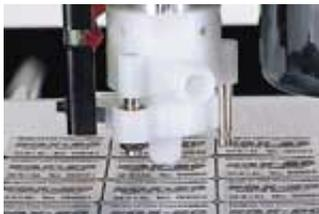
An automatic height sensor is attached to the lower end of the spindle unit. In addition to tracking the height of the material, AST controls the spindle and cutter height automatically. It also protects the surface from being scratched by cutting debris. A choice of three-different-diameter nose cones is included, allowing you to choose the most appropriate size, depending on the line thickness or curvature of the material.
